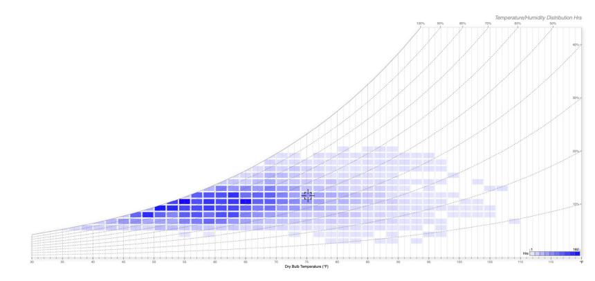
A psychrometric chart showing the frequency of ambient temperature and humidity values per year for a given location.
