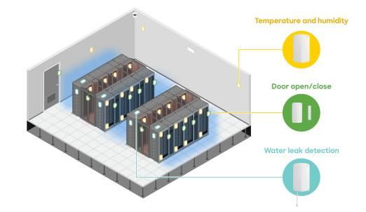
Meraki MT sensors are easy to install and integrate. By placing the sensors strategically, IT teams can reduce the complexity associated with monitoring temperature and humidity while ensuring they stay within the recommended ASHRAE temperature guidelines. Alerts can be sent to key stakeholders when sensor data deviates from the guidelines so issues are quickly remediated.
